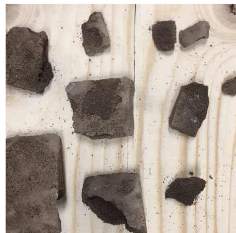
Propane nozzle did not have enough pressure. It resulted in low temperatures.
