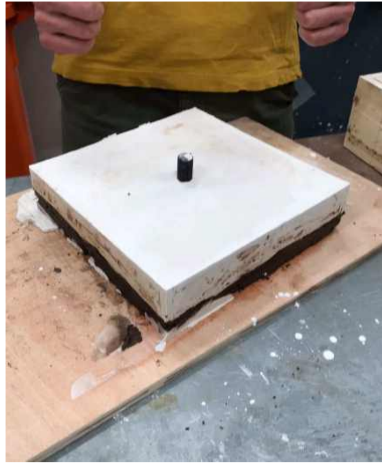
2-cover half of the mold with plaster
