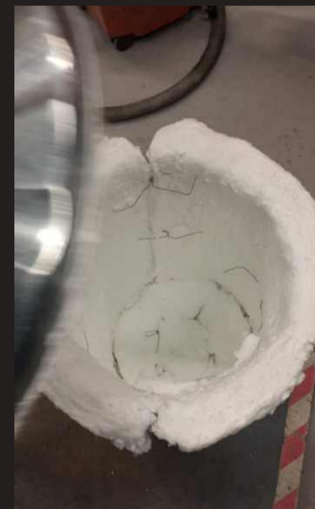
7-Leave some extra insulation on the sides.
