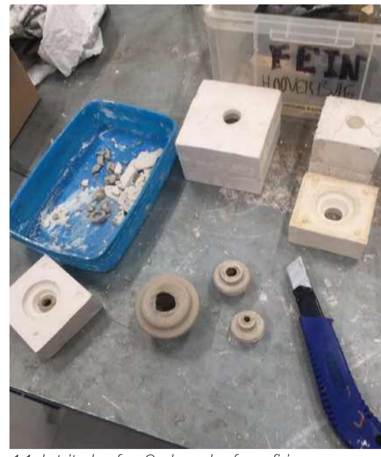
11-let it dry for 2 days before firing
