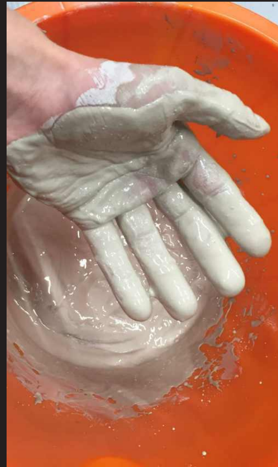
1-Make sludge around 50-50 water to clay ratio.
