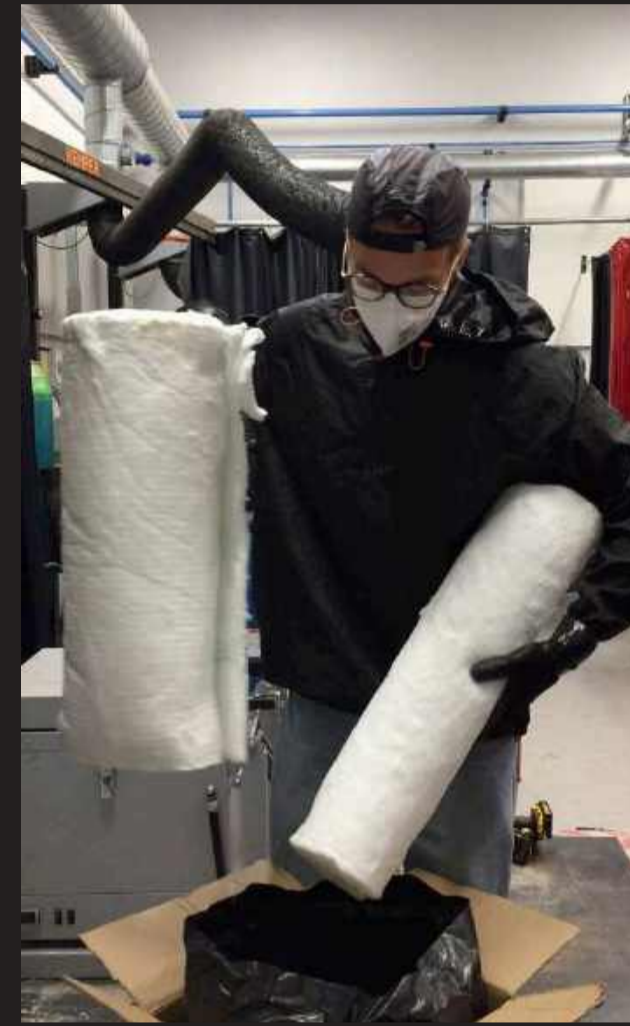
3-Ceramic insulation is toxic due to its dust particles.
