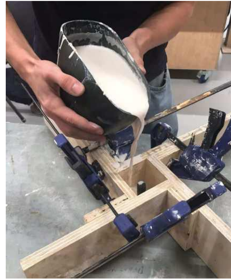
3-cover the other half with plaster
