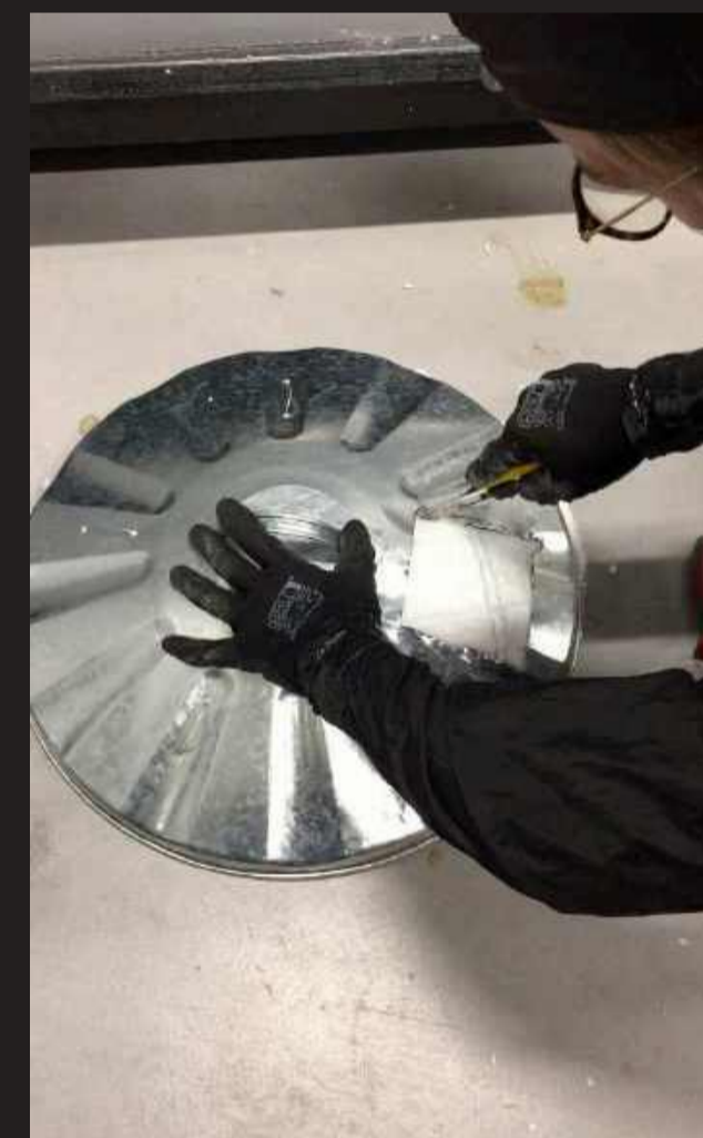
8-Make openings for inlet and outlet.
